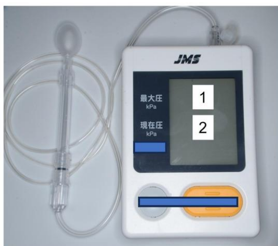
Figure 1. Device for measuring tongue pressure using an air-inflated probe. The display shows (1) peak tongue pressure (kPa) and (2) real-time tongue pressure (kPa)
